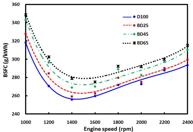
Figure 8. Brake specific fuel consumption (BSFC) with engine speed at full-load
