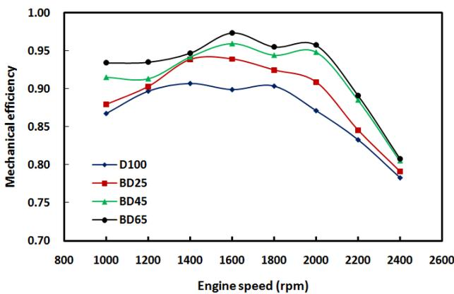
Figure 7. The mechanical efficiency with engine speed at full-load
