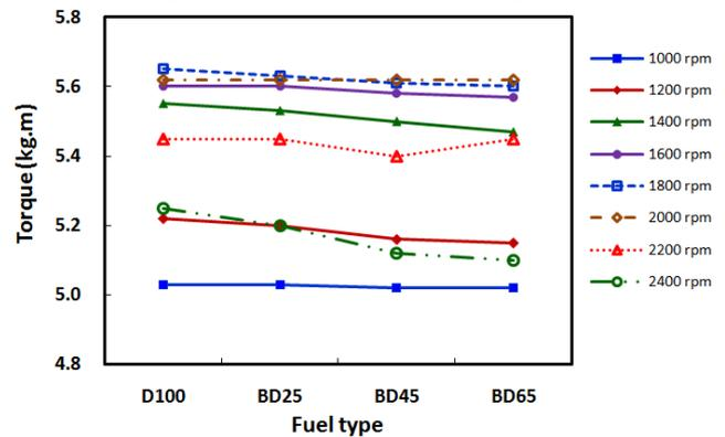
b. Torque at full-load with the fuel type
