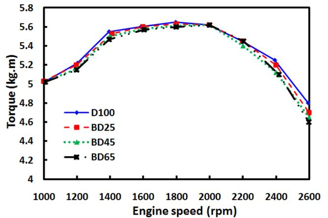
a. Torque at full-load with the engine speed
