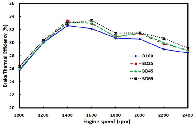
Figure 6. Brake thermal efficiency with engine speed at full-load
