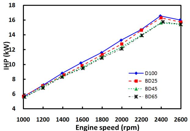
a. Indicated hp at full-load with the engine speed
