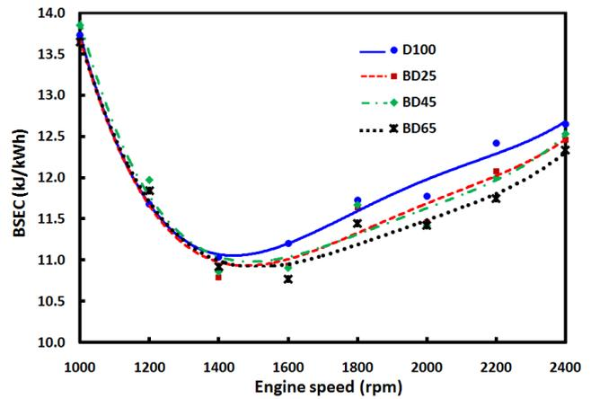
Figure 9. Brake specific energy consumption (BSEC) with engine speed at full-load
