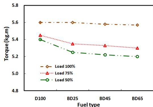
Figure 3. The torque at 1600 rpm for the various engine-loads with the fuel type
