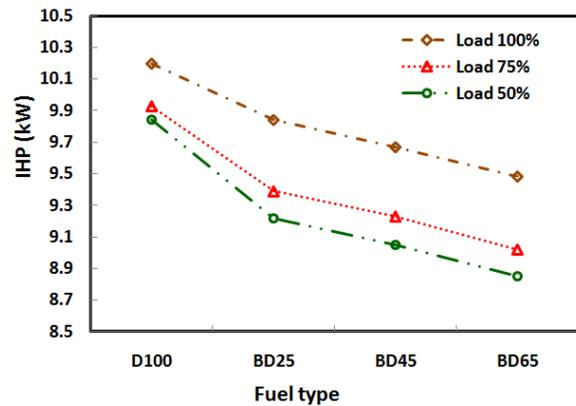
**Figure 5.** The IHP at 1600 rpm for the various engine-loads with the fuel type
