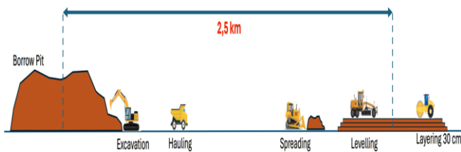
Figure 1. Cut and fill work illustration
