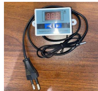
Figure 13. Temperature controller XH-W3001.
