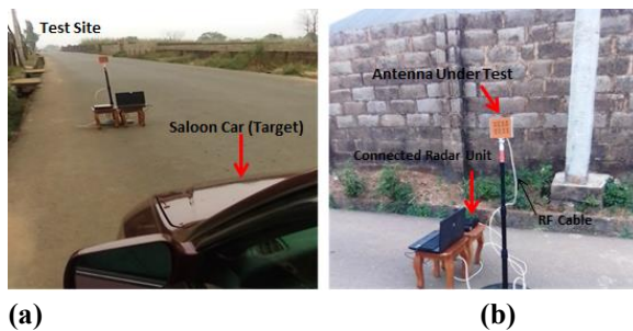
Fig. 13: Photograph of the Car Speed Monitoring Test: (a) Test Site, (b) Measurement Setup
