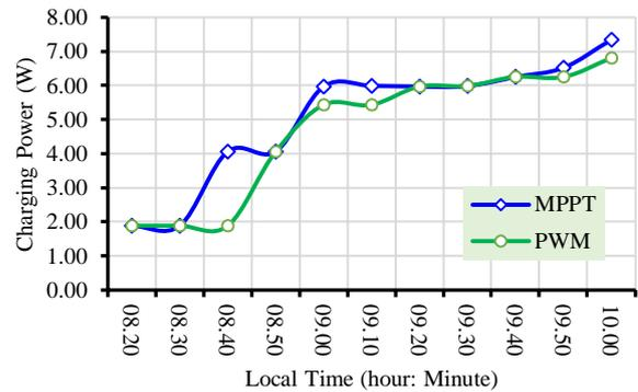
**Figure 4.** Comparison of MPPT and PWM controllers on running e-scooters.
