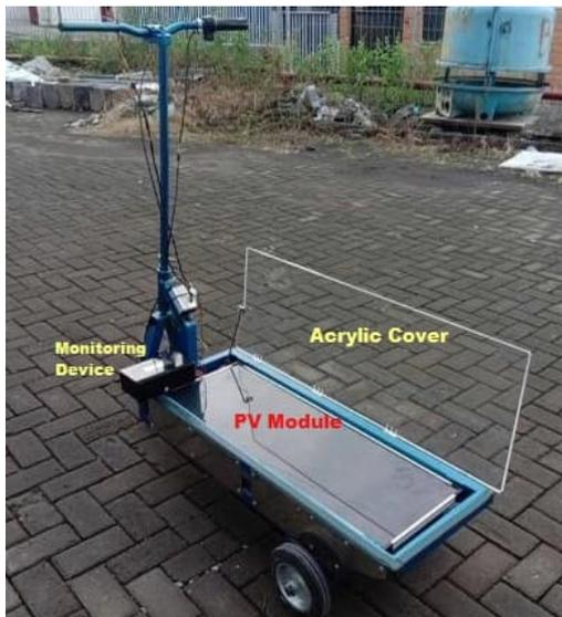
**Figure 2.** Prototype of a solar-powered electric scooter
