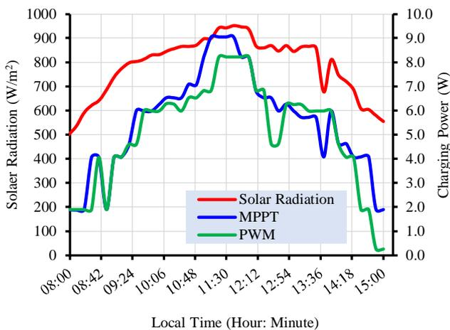
**Figure 3.** A graph comparing MPPT and PWM charging power over local time in stationary e-scooter conditions
