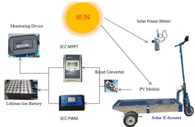
**Figure 1.** Experimental setup for comparing solar chargers on E-Scooter
