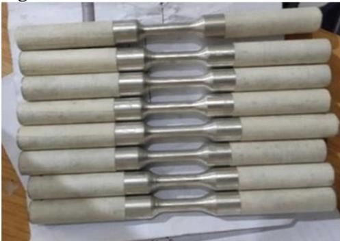
**Figure 5.** Shape of the tensile test specimen Based on the results of the tensile test that has been done
