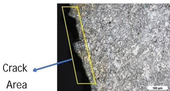
**Figure 7.** Microstructure of AZ-31B magnesium fault region
