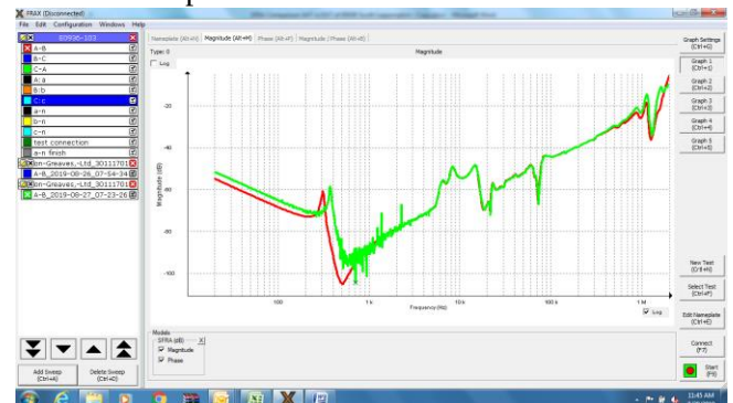
Figure 12. Comparison of SFRA FAT and SAT 2nd between HV Phase A & B
